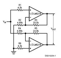
Single ended input to differential output  $A_V = 10, BW = 3.2 MHz$ 40 V<sub>PP</sub> Response = 1.4 MHz  $V_S = \pm 15V$
