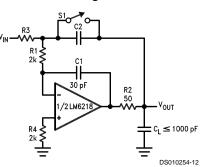
Examples of unity gain connections for a voltage follower, Inverter, and integrator driving capacitive loads up to 1000 pF are shown here. Different R1–C1 time constants and capacitive loads will have an effect on settling times.
