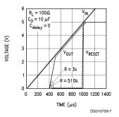
FIGURE 2. Reset Output Behavior during Power-Up
