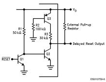
FIGURE 1. Delay Reset Output
