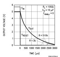
FIGURE 3. Reset Output Behavior during Power-Down
