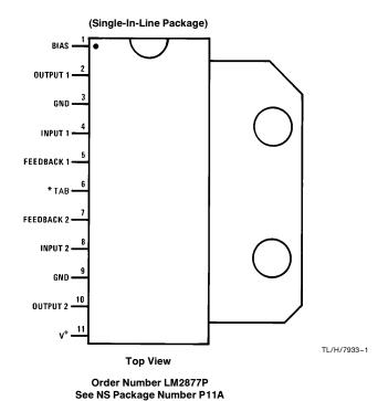
\*Pin 6 must be connected to GND.
