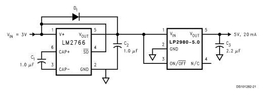
FIGURE 5. Generate a Regulated +5V from +3V Input Voltage
