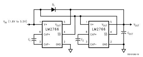
FIGURE 3. Lowering Output Resistance by Paralleling Devices
