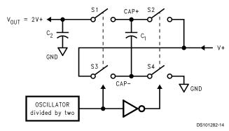
FIGURE 2. Voltage Doubling Principle
