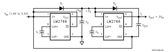
FIGURE 4. Increasing Output Voltage by Cascading Devices
