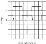
V<sub>NSW</sub> Response to SDP (with 5mA Load)
