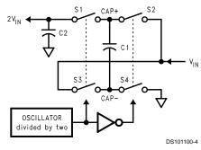
FIGURE 2. Voltage Doubler Principle
