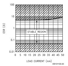
FIGURE 4. ESR Curve for  $C_{OUT} = 2.2 \mu F$
