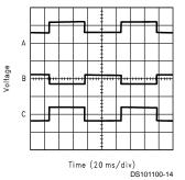
A: INPUT VOLTAGE: V\_{IN} = 3.2V to 6.0V, 5V/div B: OUTPUT VOLTAGE: VPSW: 100mV/div C: OUTPUT VOLTAGE: V<sub>NSW</sub>: 100mV/div
