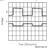
A: LOAD CURRENT:  $I_{LOAD} = 4.4mA$  to -9.4mA, 10mA/div B: OUTPUT VOLTAGE: V<sub>NSW</sub>: 50mV/div
