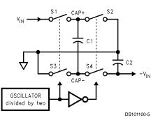
**FIGURE 3. Voltage Inverter Principle**
