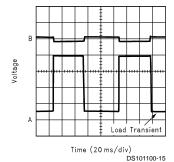
A: LOAD CURRENT:  $I_{LOAD} = 5mA$  to 39.6mA, 10mA/div B: OUTPUT VOLTAGE: V05: 10mV/div
