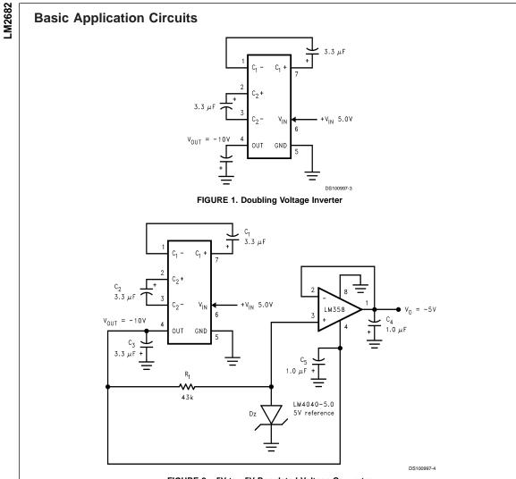
FIGURE 2. +5V to -5V Regulated Voltage Converter
