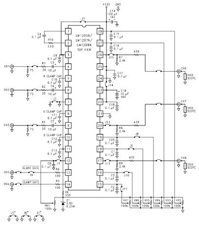
FIGURE 15. Demonstration Board Schematic
