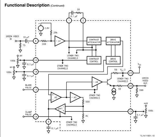
FIGURE 6. Block Diagram of LM1205 Video Amplifier
