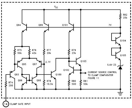
FIGURE 12. Simplified Schematic of LM1205 Clamp Gate Circuit
