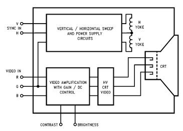
FIGURE 5. Typical RGB Color Monitor Block Diagram
