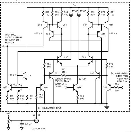
FIGURE 11. Simplified Schematic of LM1205 Clamp Comparator Circuit
