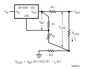
FIGURE 4. Best Load Regulation using Adjustable Output Regulator
