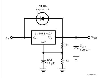
FIGURE 5. Regulator with Protection Diode
