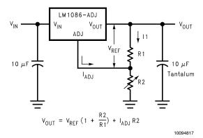
FIGURE 2. Basic Adjustable Regulator
